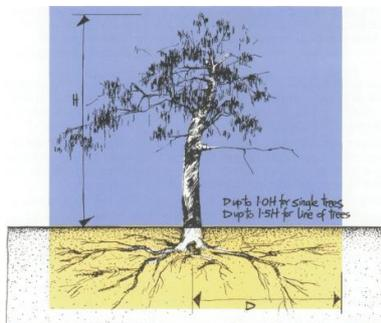
Diagram 3 on the next page shows the typical damage resulting from a large tree having been planted too close to the footings at a corner of a brick house – the tree has extracted the moisture from around and under the corner, resulting in subsidence. A tree root barrier would have restricted the spread of the roots and therefore the consequential water extraction from the soil under the footings.
